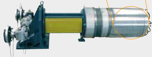
Disc Die Head with cooling mandrel
